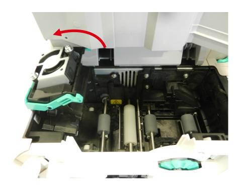
3. Use the Evolis pre-saturated cleaning card to clean the transport rollers by rotating the transport wheel. Repeat the step for each transport roller.
