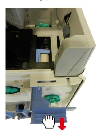
5. Rotate the flip over wheel and locate the flip over rollers as shown.
