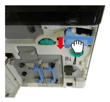
${\it 3.} \quad \hbox{Lift up the tape spindle and remove the cleaning roller}.$
