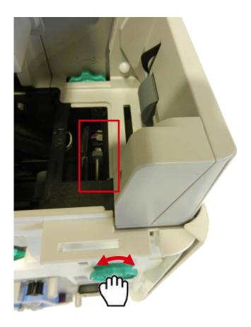
8. Insert the Evolis pre-saturated cleaning card between the flip over rollers and the white pressure rollers. Rotate the flip-over wheel to clean the flip-over rollers by keeping the cleaning card in your hand. Do not hesitate to blow with a dry air pressure spray.
