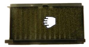
4. Use a dry air pressure spray to clean the filter.
