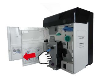
5. Insert the Evolis pre-saturated cleaning card between roller and the chassis. Clean the nip roller surface with the pre-saturated cleaning (a) by rotating it with a flat screwdriver (b).
