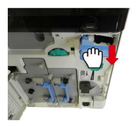
4. Remove the cleaning tape cassette handle, lift it and pull.
