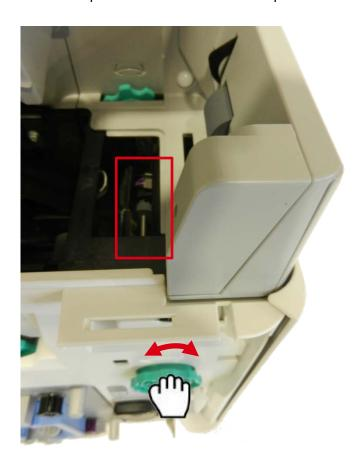
6. Insert the Evolis pre-saturated cleaning card between the flip over rollers and the white pressure rollers. Rotate the flip-over wheel to clean the flip-over rollers by keeping the cleaning card in your hand.
